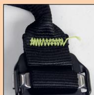
End of thread loose
