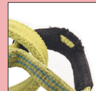
Abrasion protector worn
