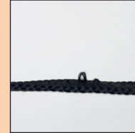
Loop pulled on smooth webbing
