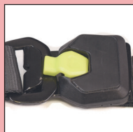
Triple Lock buckle with broken button
