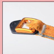
Webbing worn at buckle
