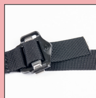
Webbing termination missing
