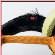
Abrasion protector worn, indicator visible
