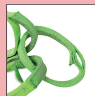
Open general stitching enables misuse
