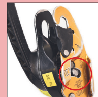
Rivet has excessive play
