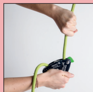
System does not block when pulled suddenly
