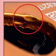
Dents in the gear due to intense falls
